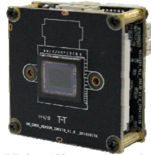
38 board, 5MP low illumination and power consumption and code stream. IR-CUT drive, 3D noise reduction, H.264/H.265 solution
