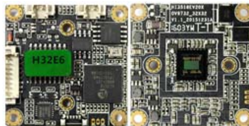
32 single board, 1MP, low illumination and power consumption and code stream. IR-CUT drive, 3D noise reduction, H.264
