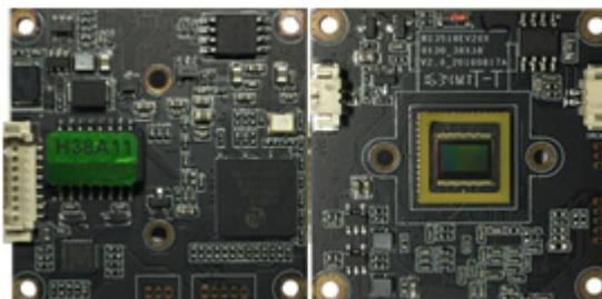
38 single board, 2MP, low illumination and power consumption and code stream. IR-CUT drive, 3D noise reduction, H.264+
